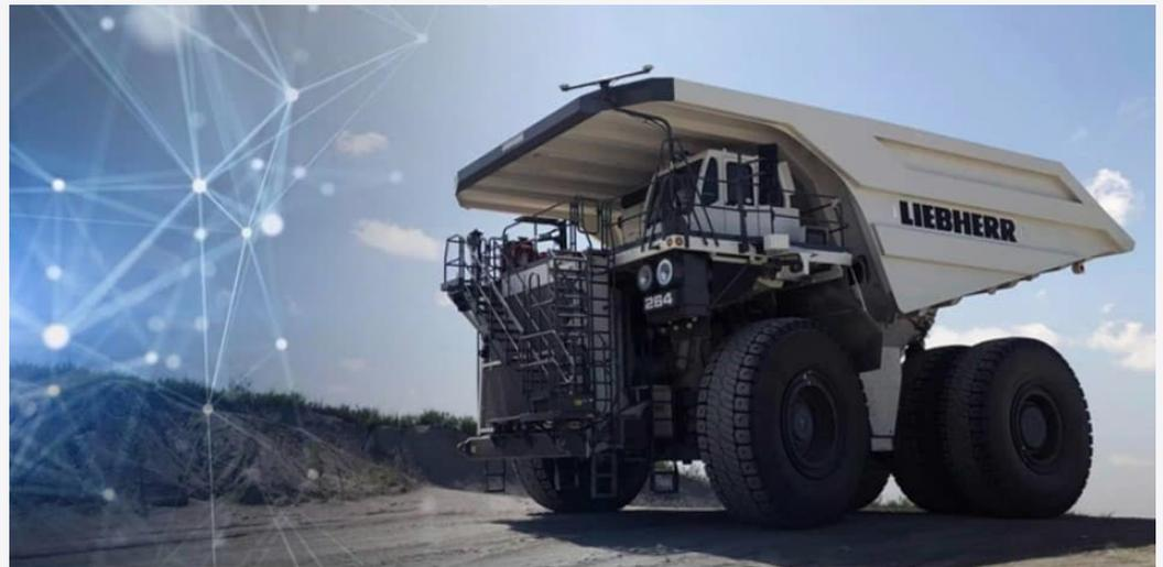
Liebherr 240 tonne mining truck; 1.4MWhr battery; 30 minute charging
