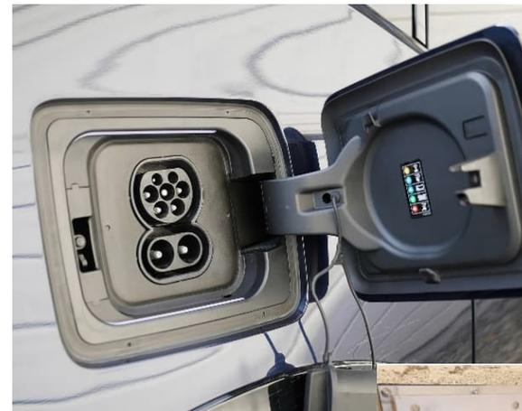
CCS type 2 as used to charge batteries in vehicles.
