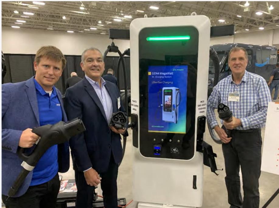
Prototype BTC Power SAE J3271/SAE J3400 dual output charging station.
