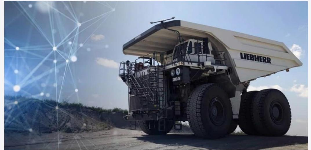
Liebherr 240 tonne mining truck; 1.4MWhr battery;
