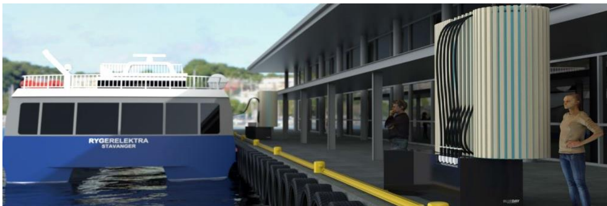
Figur C.2 – Blueday parallelle CCS2 tilkoblinger
