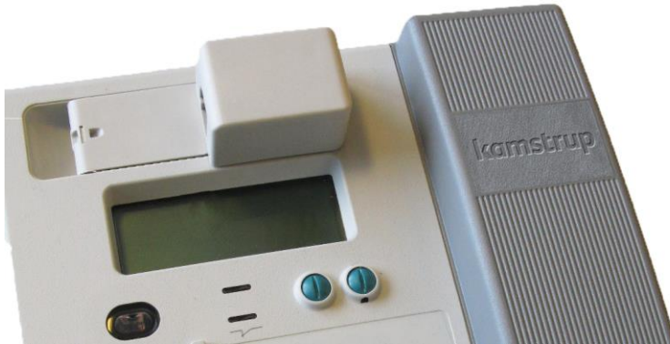
Figure 1: Kamstrup OMNIPower meter with HAN-NVE interface module.
